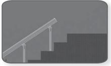
**Step 5:** To mark the location for the upper guide rail, measure from the leg base plate up the wall 36.25" (as indicated by the red vertical line). Be sure to measure in the center of the leg and use a 3 or 4' level to help ensure that the measurement is plumb vertically.
