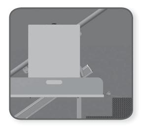
**Step 21:** Turn on the main power breaker on the chassis. The status LED indicator will cycle from RED to AMBER to GREEN to OFF, and then the lift will emit a beep. The indicator should then return to GREEN, indicating the lift is now ready to run.
