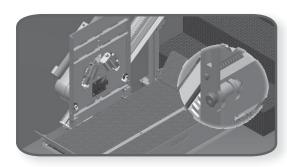
**Step 13:** Fold the platform up and attach the ends of the assist struts using the clevis and cotter pins.
