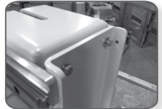
Secure the rear of the slider rails to the rear seat support using the two (2) socket bolts.
