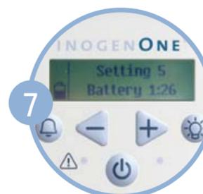
7 Set the flow setting to the flow rate prescribed by your clinical professional. The flow setting can be changed by pressing the triangular flow setting buttons that are marked with "+" and "-" symbols. Position the nasal cannula on your face and breathe normally through your nose.
