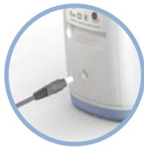
Plug the Universal Power Supply power output cord into your Inogen One G2 and position your Inogen One G2 securely inside the car. Operate your Inogen One G2 as normal.
