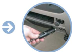
Plug the Universal Power Supply into the cigarette lighter or auxillary DC power supply.
