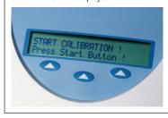
Note for those testing with Chemstrip 5 OB or Chemstrip 7 Test Strips: This calibration step is not necessary. The instrument calibration is performed automatically via the gray reference field on the test strip tray.
