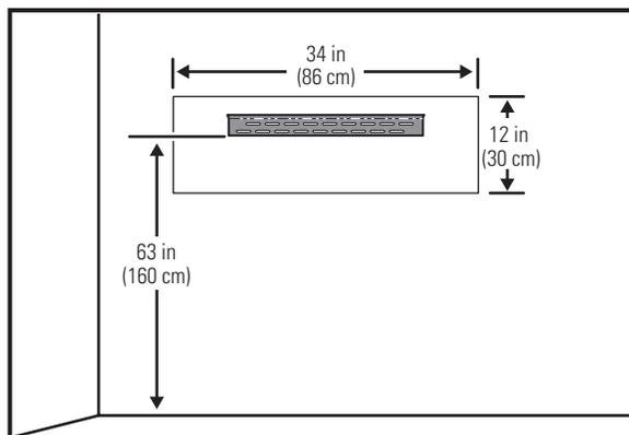
3. Affix the mounting rail bracket to two studs at the selected height using the available screws (anchors are provided for additional support).
