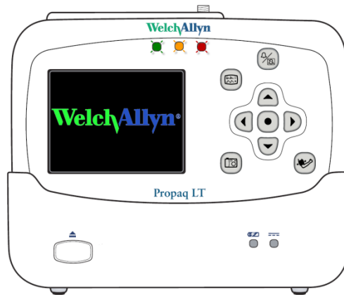
Propaq LT in Update (Bootcore) Mode with Front LEDs Flashing
