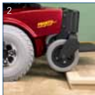
1. Center-Wheel Drive 2. Simplified Invacare® SureStep® Suspension
