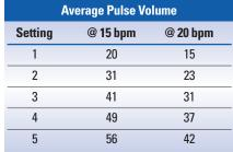
The patented, integrated electronic conserver provides a substantial bolus of oxygen at each setting and breath rate.
