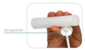
Since the internal diameter of the pressure tubing is 1.5 mm, the cross-sectional area is 1.77 mm2. The amount of air entering the flow transducer's measurement pipe during the expiration amounts to
