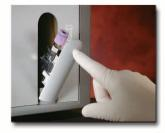
2. Place sample or control tube into the closed vial sample station
