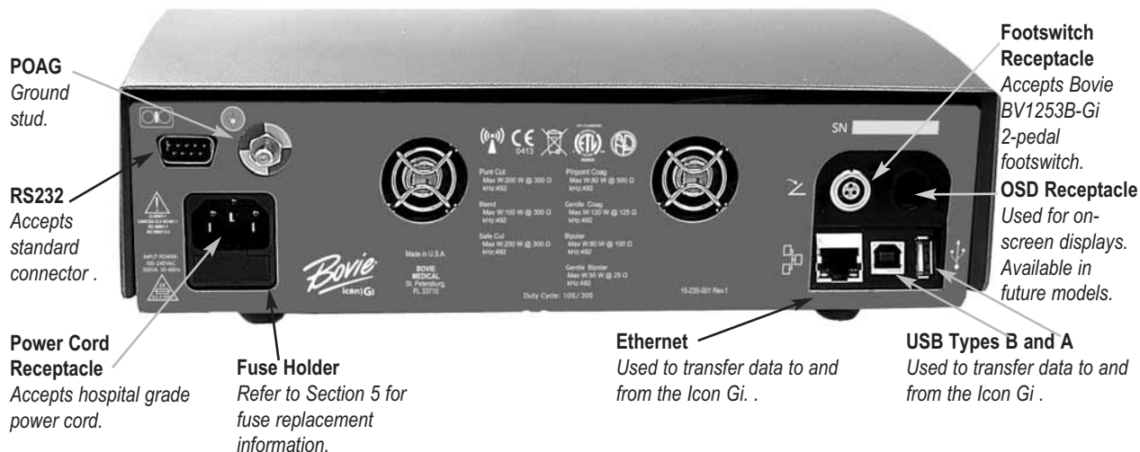
Figure 2 – 2 Layout of receptacles on the rear panel
