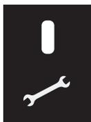
The Service LED lights up when the AED detects an error that cannot be corrected by the self test. Contact Cardiac Science Technical Support (see [Contact information](#) on page 1-2) or outside the U.S., your local Cardiac Science representative.
