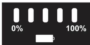
The Smartgauge Battery Status Indicator has five LEDs, four green and one red. The right four green LEDs display the remaining capacity of the battery much like a fuel gauge. With use, the green LEDs gradually go out,
