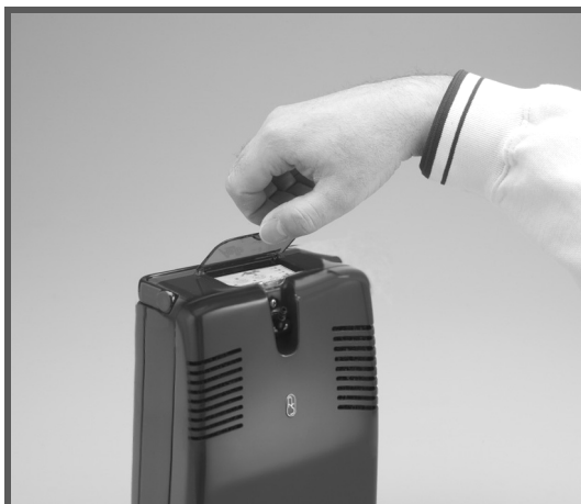
Figure 16: Lifting Dust Cover on Keypad Display
