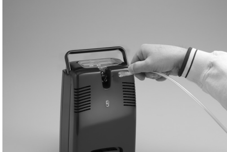
Figure 10: Connecting Cannula to FreeStyle 5's Oxygen Outlet
