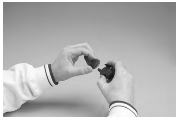
Figure 22: Removal of Filter from Filter Cover
