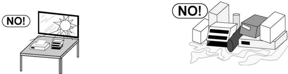
Do not place the MV1 directly in front of a heating or cooling vent. Such a location will subject it to sudden temperature changes, which may result in unstable weight readings.
