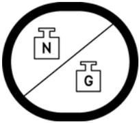
This is the **NET/GROSS** key. It is used to toggle between Net and Gross weight modes. The selected mode is indicated by turning on the appropriate annunciator on the display. Note that if no valid tare weight has been entered; pressing this key will cause (No Tare) to be shown in the 14-segment display.
