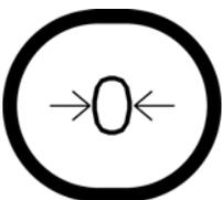
This is the **ZERO** key. It is used to reset the display to zero up to the selected limit of either 4% or 100% of the scale capacity. The zero limit is set during setup and calibration of the MV1.
