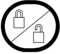
This is the **LOCK/RELEASE** key. It is used to lock and unlock the display. If the HOLD feature was enabled during setup and calibration, pressing this key (after obtaining a stable weight) will cause the MV1 to lock onto the weight. Pressing this key again will unlock the display and return it to zero.
