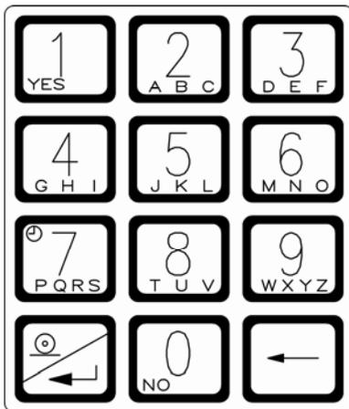
These keys are used to enter alphanumeric data during the setup and calibration as well as during normal operation of the MV1.
