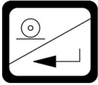
This is the **PRINT/ENTER** key. It serves several purposes. First, it is used to signal completion of the data entry and causes the MV1 to process the data entered. Second, it is used to initiate the transmission of weight and associated data using the selected I/O port.
