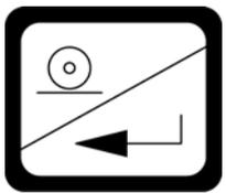
If at the menu level, this will take you to the first parameter in the currently displayed menu in the list below. If at the parameter level, this will store the currently displayed value for that parameter and proceed to the next parameter in the list below, which may depend on a [parameter condition].
