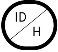
If at the menu level, this will take you to the previous menu item in the list below. If SCALE is currently displayed and the setup has been accessed through the calibration switch, then this will return you to TIME SETTINGS. If setup has been accessed through setup review, then pressing this when SYSTEM is displayed will return you to TIME SETTINGS. If at the parameter level the exact item this takes you to may depend on a [parameter condition].
