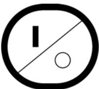
This is the **ON/OFF** key. With the MV1 off, pressing this key will apply power to it and turn on the display. If the MV1 is already on, pressing the key will turn it off.
