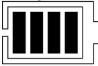
A battery status symbol will be displayed when batteries are installed. The number of bars indicates the level of charge remaining in the batteries.
