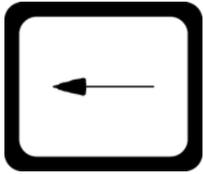
This is the **CLEAR (BACKSPACE)** key. It is used to clear an incorrect entry from the display without processing the data. If an incorrect entry is made, press this key and re-enter the correct data. When entering the ID, pressing this key will act as a “backspace” key (it will back up one space and delete the character in that space). **NOTE:** The **CLEAR** key must be pressed before the **PRINT/ENTER** key to ensure the data is not processed.
