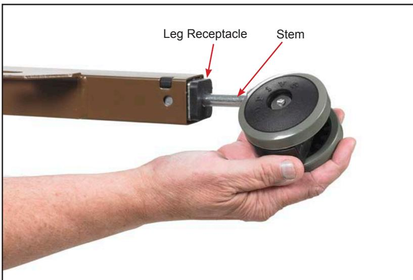
9. Install the casters by inserting the stem of the caster into the leg receptacle. It is recommended to install 1 locking caster and 1 non-locking caster on each bed end. The locking casters should be installed diagonally from each other.
