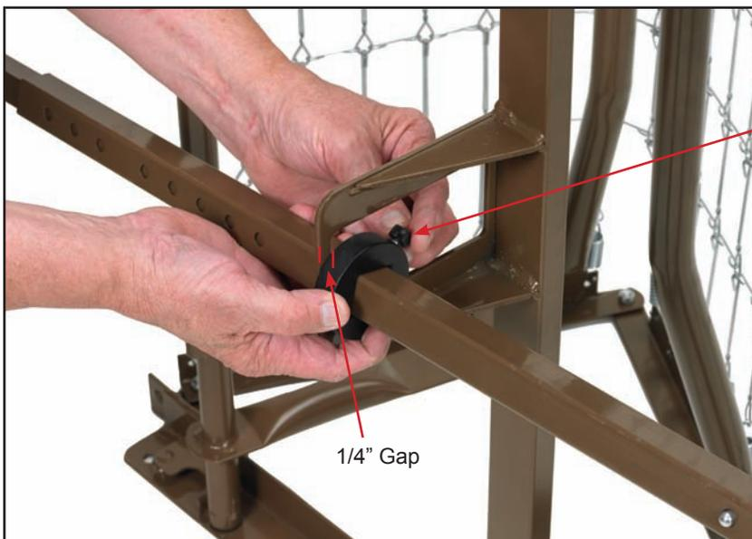
6. Slide lock collar 1/4" from the foot side of the hanger bracket as shown. Tighten thumb screw.
