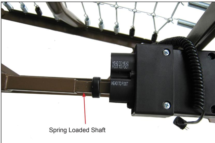
5. Install Hi/Low shaft to the Hi/Low motor at the foot section of the bed by inserting the spring loaded side of the shaft to the bottom receptacle as shown.
