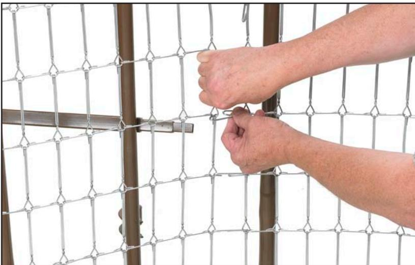
8. Connect head section and foot section by squeezing together and attaching with spring links. Pull up the head section and foot section to release tension between the springs.
