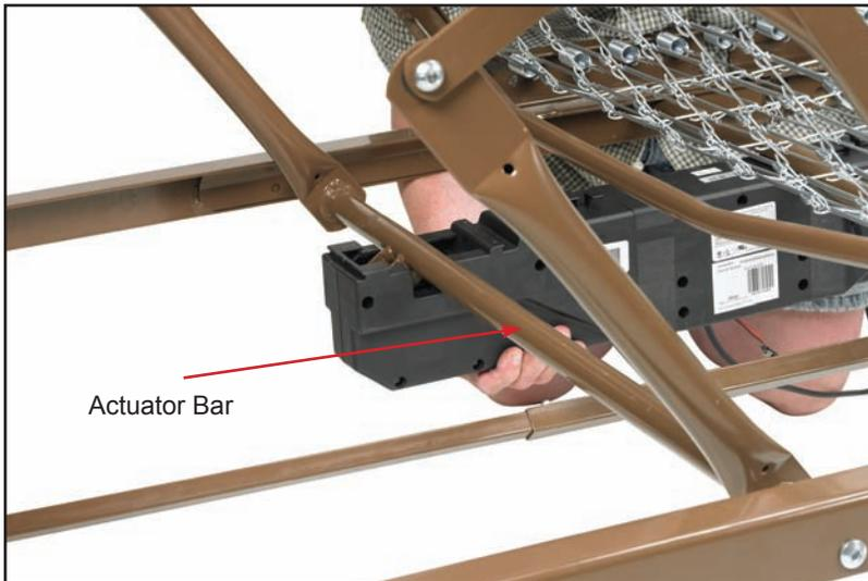
16. Align the motor with the actuator bar and lift the head spring to the highest position. The motor will automatically be pulled towards the bed and lock onto the actuator. Repeat for foot section.
