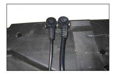
NOTE: Before installing motor, plug hand pendant and Hi/Low motor cable into motor as shown
