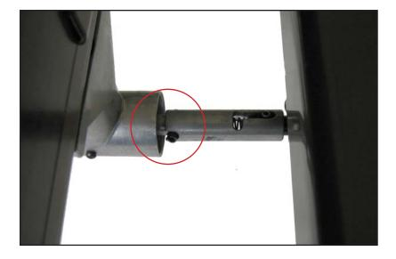
14. Make sure the slot on the spring loaded shaft engages the roll pin on the gear box.
