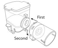
· Place the container with fitted mesh firmly onto the housing or base of the device, until you hear it click into place on the left and right.
