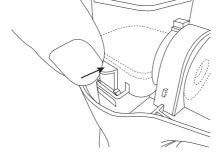
• Remove the medicine container and mesh nebulizer by pressing both brackets inwards and drawing the device out.
