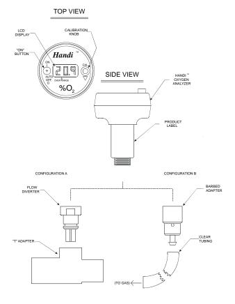
**LCD Display:** A 3-digit display provides a direct readout of oxygen concentration in the range of 0 - 99.9%. The display is blank when the *Check and Go Disposable* enters its Sleep (power off) mode. The *Check and Go Disposable* will automatically enter the Sleep mode after approximately 1.3 minutes from the last time the ON button was pressed.
