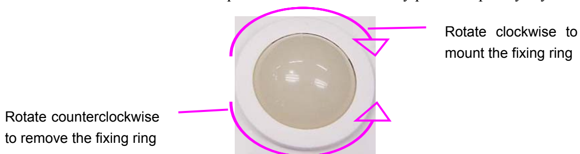
Figure 13-4 Assembling and Disassembling Trackball
