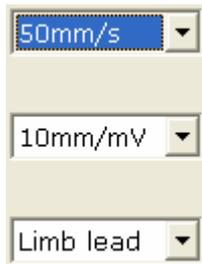
You can set the speed and the gain of the displayed ECG waves. The lead number and the lead type of the displayed ECG waves can also be chosen.
