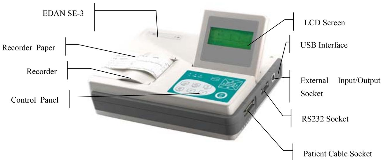
Figure 2-2 SE-3 (192×64 dot single color LCD screen, hereinafter called SE-3 Narrow screen)
