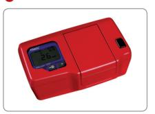
Within 90 seconds, the result is displayed in mg/L. Record the result. The result will remain on the display until the lid is opened. If the display shows:
