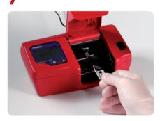
Open the lid and discard the used cuvette. Close the lid. When the display shows the the HemoCue symbol and three flashing dashes, the analyzer is ready for a new measurement. When the measurements for the day have been completed, switch off the analyzer with the ON/OFF button
