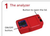
Make sure that the analyzer lid is closed. Press and hold the left button until the display is activated. The display shows the version number and an internal quality control, the "self test" is performed. Three flashing dashes are displayed when the analyzer is ready for use.
