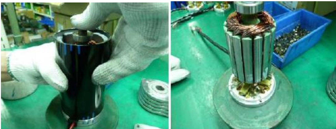
Step 5: Use the right hand to press the wire winding. Use the left hand to remove the outer tube from the wire winding.
