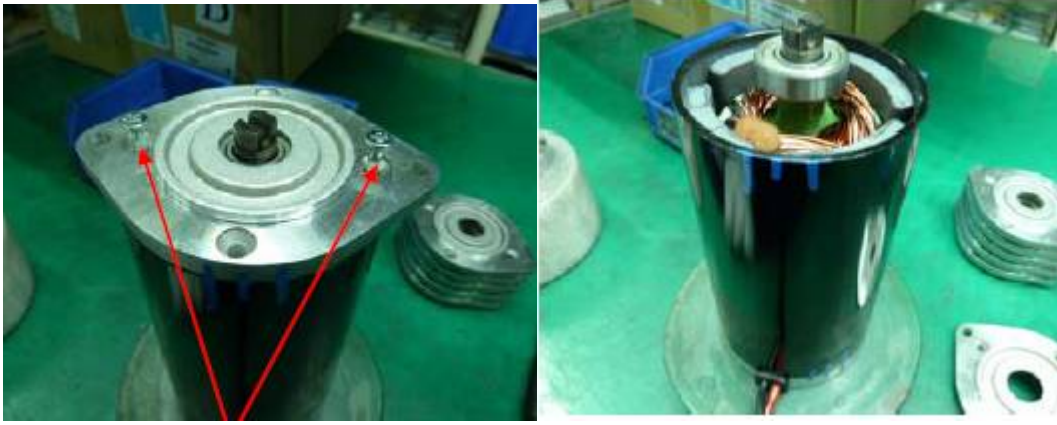
Step 4: Loosen two units of screws properly and then remove the front bracket.
