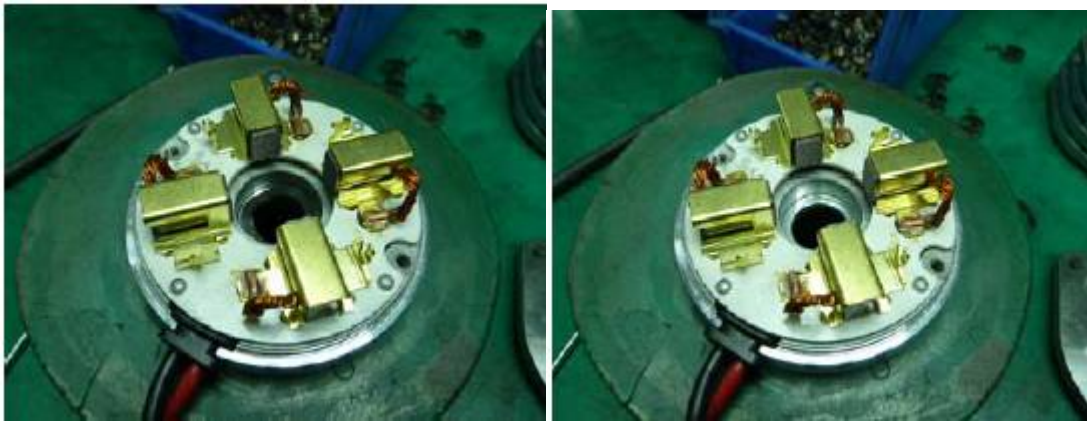
Step 7: Remove the brush springs and remove the wave-shaped pad
