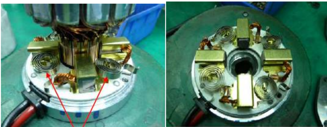
Step 6: Pull those 4 units of brush spring and then remove the wire winding
