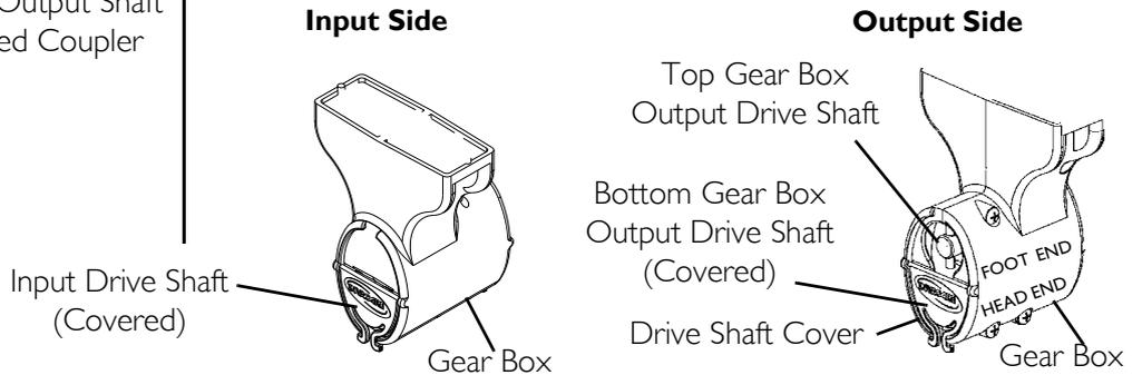
**FIGURE 10** Assembling/Installing/Removing Drive Shaft
