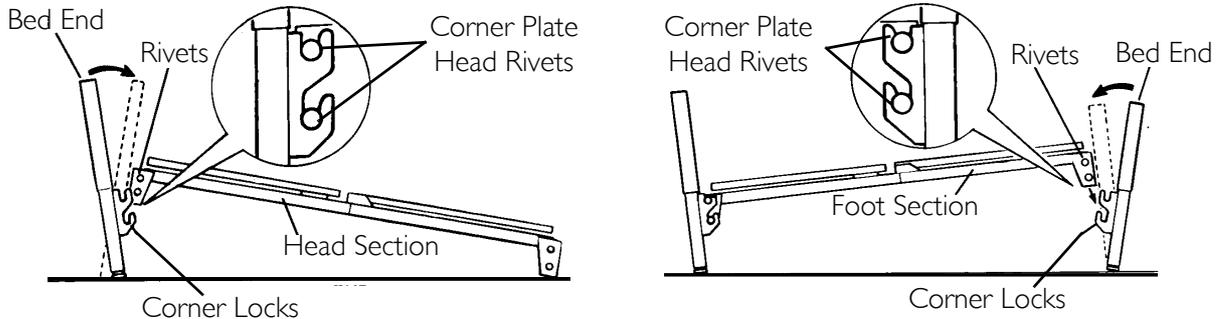
**FIGURE 5** Installing/Removing Bed Ends
