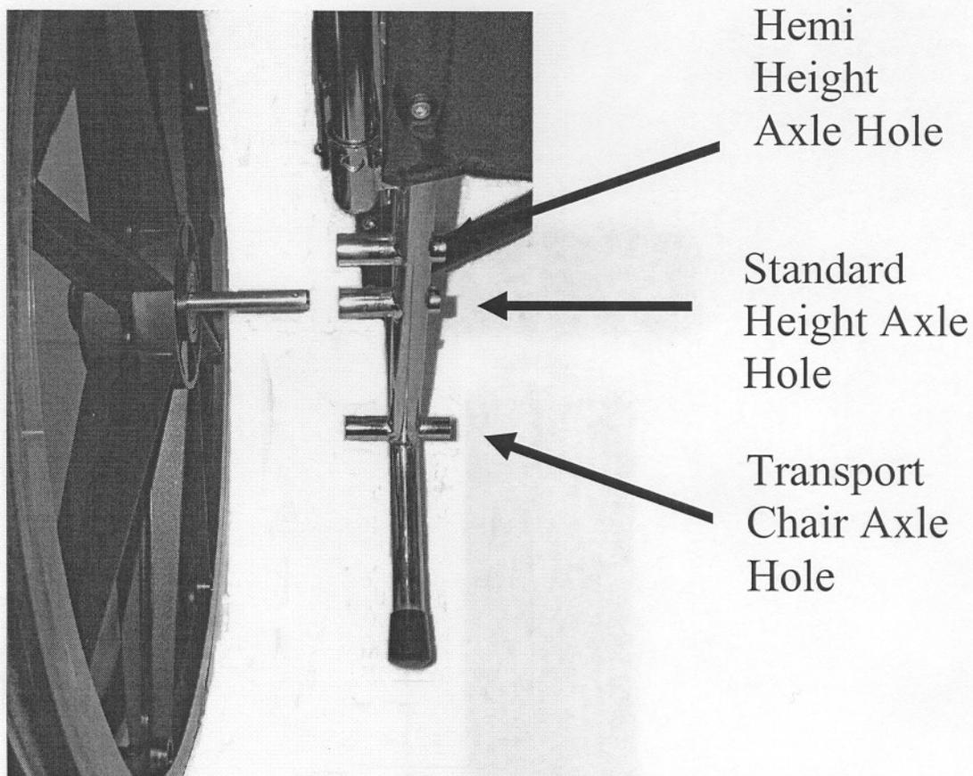
**Step 1:** Depress the quick release button on the wheel hub and pull off the wheel and quick release the axle from the standard height axle hole.
