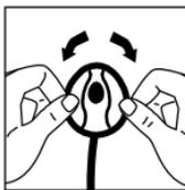
With the diaphragm side up, push the rim at one point with both thumbs and roll the rim off the edge of the chestpiece. Remove the diaphragm from the rim and clean parts in soapy water or wipe with alcohol. Wipe chestpiece surfaces with alcohol or soapy water. Dry all parts and surfaces thoroughly before reassembly.
