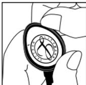
To attach the rim/diaphragm assembly to the chestpiece, engage the groove of the rim (with the diaphragm attached) around the chestpiece at one point and hold it in place with your thumbs. Slowly roll the rim around and over the chestpiece edge using
