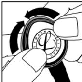
examine the ring to ensure that the flexible edge is smoothly engaged inside the rim. Refer to illustration for correct assembly of the non-chill rim and diaphragm. If necessary, flex the assembly by pinching the outer rim edge between the thumb and fingers.
