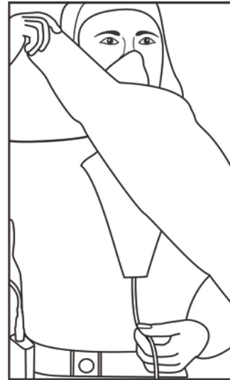
Fig. 6: Routing cable beneath inner shroud.
