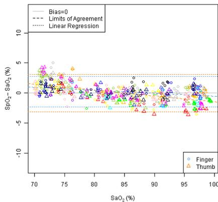
This graph shows plots of the error (SpO<sub>2</sub> – SaO<sub>2</sub>) by SaO<sub>2</sub> using the 9590 with a linear regression fit and upper 95% and lower 95% limits of agreement. Each sample data point is identified by subject from a clinical study in non-motion conditions.
