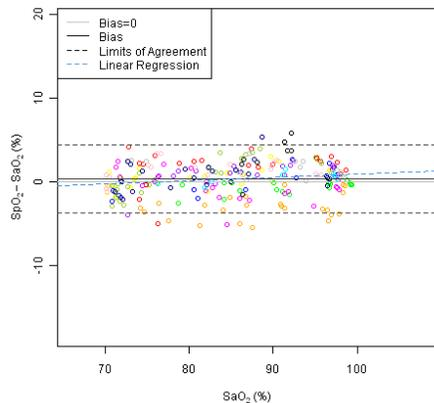
This graph shows plots of the error (SpO<sub>2</sub> – SaO<sub>2</sub>) by SaO<sub>2</sub> using the 9590 with a linear regression fit and upper 95% and lower 95% limits of agreement. Each sample data point is identified by subject from a clinical study using toes in non-motion conditions.
