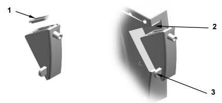
Figure 6. Replacing the Moisture Trap/Filter
