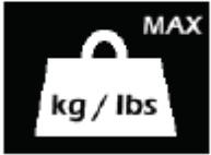
If the lift stops because of overload, the symbol will appear on the display and give user the information about why the lift is stopped.
