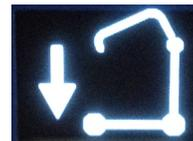
The display showing a lifting actuator is moving down.
