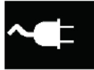
If someone tries to use the lift while mains plugged in, the symbol will appear on the display. The user receives the information about why the lift is not working. Usage of lift while charging is not possible.
