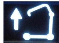
The display showing a lifting actuator is moving up.
