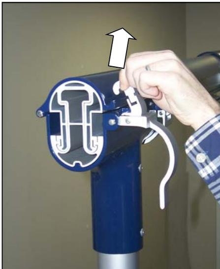
Once the Latch is lifted up and away from the Track Holder Lid it can be released. Repeat this procedure for each of the Latches.
