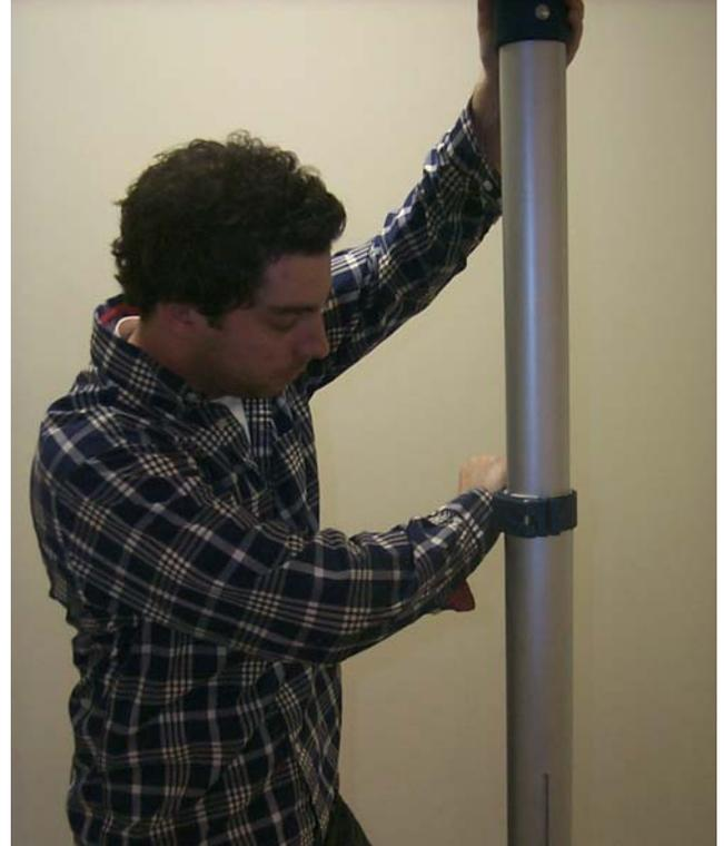
Photo showing the position of the locked Post Clamp. It must fit snugly against the Bottom Post Section.
