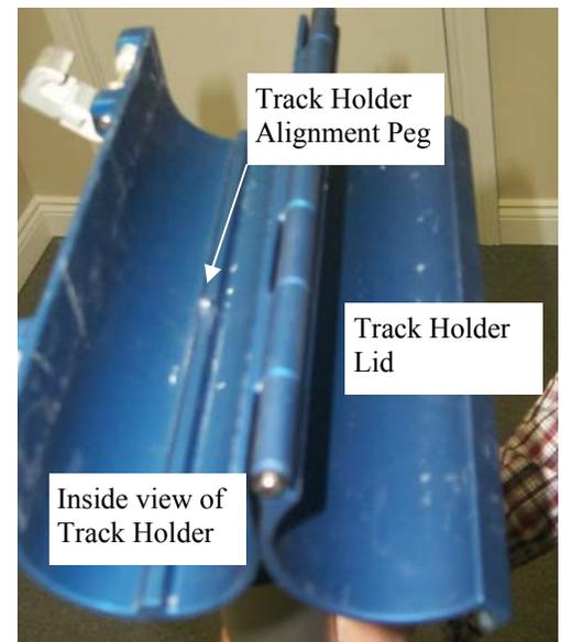
Photo showing inside view of Track Holder with the Track Holder Lid open. On the bottom of the Track Holder is the Track Holder Alignment Peg.
