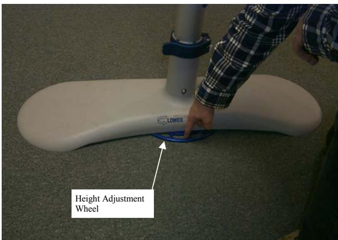
Photo showing close-up of Height Adjustment Wheel. Turn the wheel either to the left or right to make small adjustments to the height of the track. Use the Height Indicator and Ruler to make sure that both sides of the Side Support Assembly are at the same height. This will ensure that the Adjustable Track is level and safe for use. For multi-level setting refer to the section of this manual titled "Multi-Level Set-Up".
