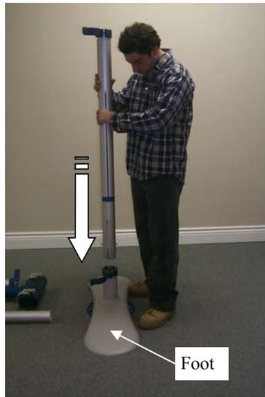
**Step 2** - With the Foot Clamp Arm swung in a open position, place one of the Lower Post Section pieces securely into the open hole of a Base piece. Ensure that it is pushed all the way in.
