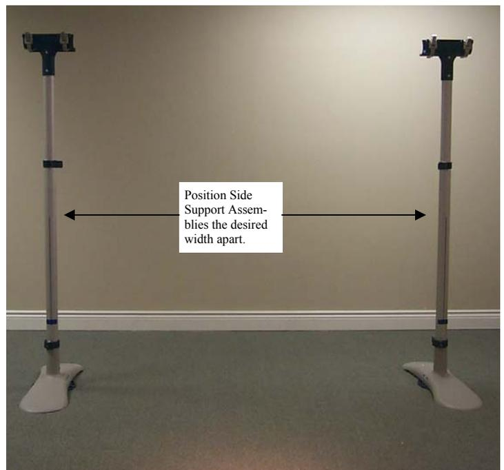
**Step 11** - Proceed to set up the second Side Support Assembly by following the steps 1 - 10. Carefully move both assemblies to their final location. Be sure that the Track Holders are roughly aligned together. This will make placement of the Adjustable Track easier to accomplish.
