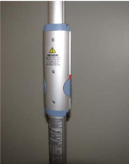
**Safety Lock and Level must be firmly Engaged in housing.**
