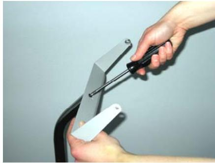
5. Use the two stand mounting knobs to attach the mounting bracket to the Vista **ABI**.
