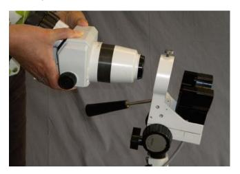
Caution: Do not tilt head all the way back as eyepieces can slide out of the binoculars and become damaged.
