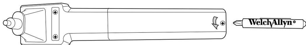
2. Remove the battery cover by lifting the bottom of the cover away from the probe tip.
