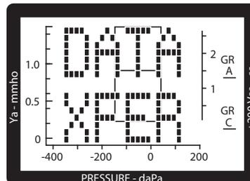
When the DATA XFER message displays, the device has made the data connection to the Printer/Charger. Any 226-Hz data stored in the Handle is now available for printing.
