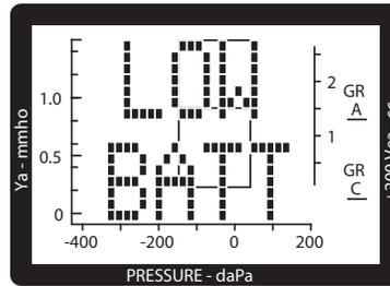
The LOW BATT message indicates that the battery needs to be recharged. The system will not perform a test in a LOW BATT condition. All buttons are disabled to prevent inaccurate results due to inadequate battery voltage. Normal operation may be restored by recharging the battery or replacing the battery with a charged battery. Stored data is not lost when the battery is removed.
