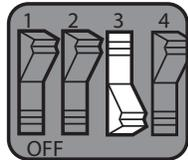
Depress the ON portion of the switch to select this option. Only the tympanogram and the GR (Width) numeric value will print.
