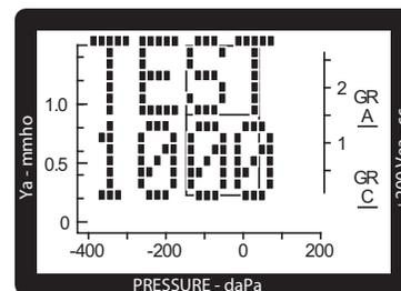
The TEST message indicates that the test has started. Test data will begin to appear immediately.
