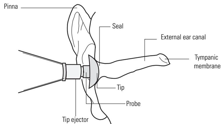
2. Push the tip onto the probe, making sure that the tip is fully seated.
