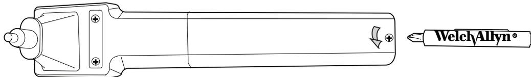
3. Remove the battery cover by lifting the bottom of the cover away from the probe tip.
