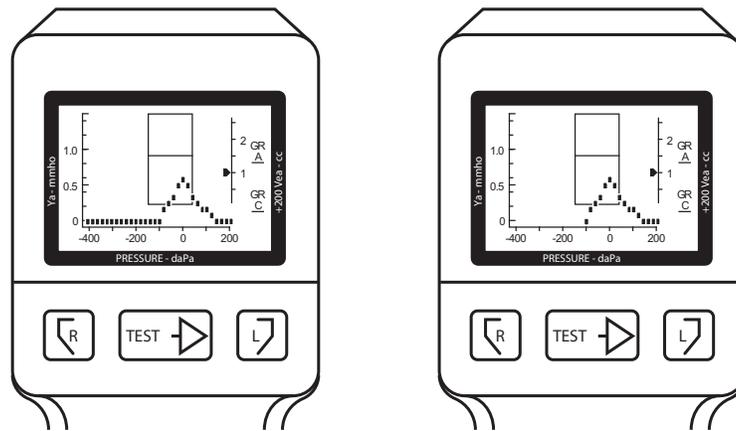
For 1000 Hz, the test is complete when one of two “Quick-Interpretation” messages appears—either PASS or REFER—as shown in the examples below. If patient or instrument movement causes a leak beyond -300 daPa in 1000-Hz mode, the test will be stopped but the data will be saved.
