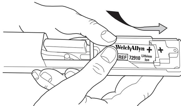
4. Replace the cover by inserting the tip end under the front cover, lowering the opposite end, and replacing the screw.
