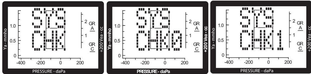
The SYS CHK (SYS CHK0, SYS CHK1) message indicates that the Handle is doing a self-check to ensure proper operation. The Handle will shut off upon completion of the test. Press any button to power the Handle and clear the condition.
