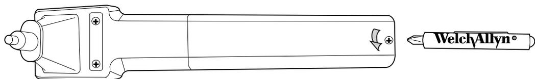
3. Remove the Handle cover by lifting the bottom of the cover away from the probe tip.
