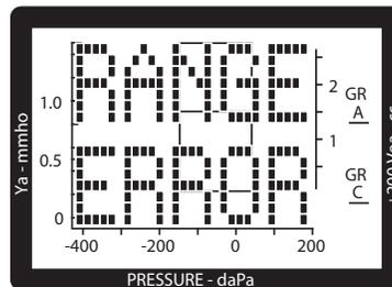
The RANGE ERROR message indicates that a large pressure change occurred during a test. If this message appears, press the TEST button and start the test again.
