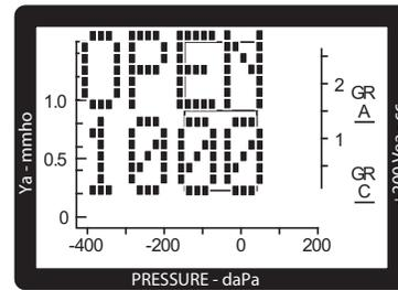
The test has not begun since a valid ear cavity has not been detected.
