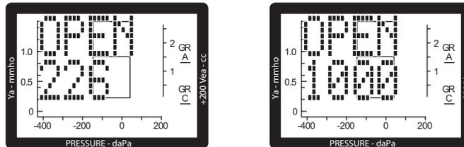
**Note** The default frequency set at the factory is 226 Hz. To change the default frequency to 1000 Hz, see the instructions at the end of this chapter.
