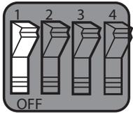
Depress the OFF portion of the switch to select this option. This causes the printout to begin only when the PRINT button is depressed.
