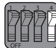
This switch is used during manufacturing only. Leave this switch in the OFF position. The Printer/Charger will not operate normally if this switch is on.
