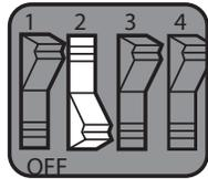
Depress the ON portion of the switch to select this option. This causes messages which interpret the tympanogram to not be included on the printout.
