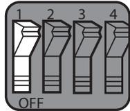
Depress the OFF portion of the switch to select this option. This causes the messages which interpret the tympanograms to be included on the printout.
