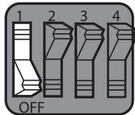
Depress the ON portion of the switch to select this option. This causes the printout to begin automatically once the Handle is placed in the well, and data transfer is complete.
