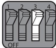
Depress the OFF portion of the switch to select this option. Both the tympanogram and its corresponding numeric data will print.
