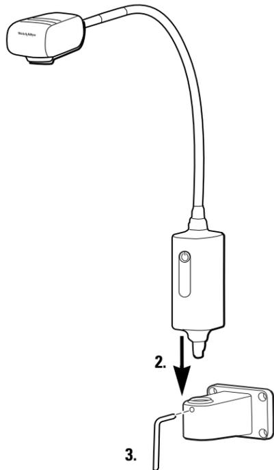
**WARNING:** Ensure that the mounting bracket is securely anchored to the wall or table, or that the mobile stand is securely assembled, and the exam light is securely fastened to the bracket or stand as directed. Do not hang or place objects on the equipment.
