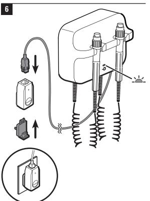
Attach Welch Allyn 3.5V instrument heads of your choice to the handles. See the directions for use for each instrument head.
