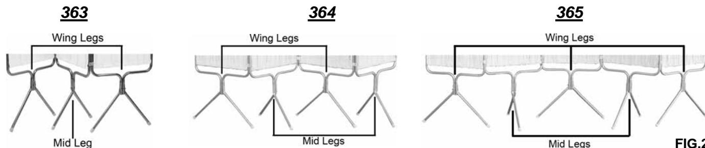
2. Check screen for levelness, if necessary the legs can be gently bent so that all legs touch the floor.
